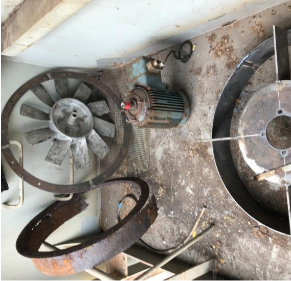
Cropping and renewal of C/H ventilation casing were carried out on board.
